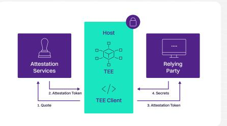
Remote attestation is the main technical mechanism to allow a remote entity to verify the code running in a TEE, by validating the signed measurements of the code computed by the root of trust on the CPU, using a key that is unique to the hardware.
